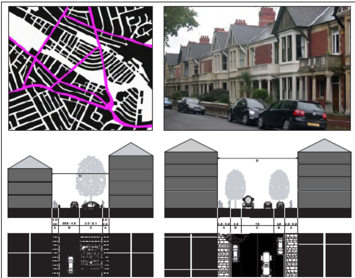
ABOVE: STREETS CAN BE GIVEN DIFFERENT CROSS SECTIONS TO EXPRESS THEIR RELATIVE IMPORTANCE IN TERMS OF BOTH MOVEMENT AND URBAN STRUCTURE STRENGTHENING LEGIBILITY
